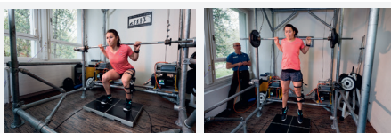
Fig. 1 & 2: Measurement of the bilateral isometric squat in the low position with 70° knee flexion on the force plate with a fixed bar. Explosive strength test with additional load.
